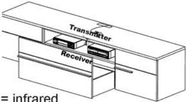
The IR repeater passes signals from standard IR remote controls into the unit. A DVD player can therefore be operated from behind a closed front, for example. Incoming IR signals are received by the receiver and passed on inside the unit via the transmitter. The repeater does not require its own remote control. A 220-volt mains connection is required for operation.<br>IR = infrared |
