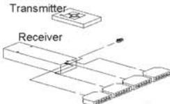
A maximum of four power circuits can be switched and dimmed using the remote control. Six light fixtures can be included in each power circuit. If required, the remote control is connected between the transformer and lighting.                                                                                                                                                                  |
