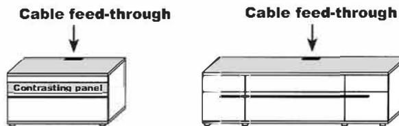
The cable feed-through has a flap and a sealing brush to guide cables easily.
